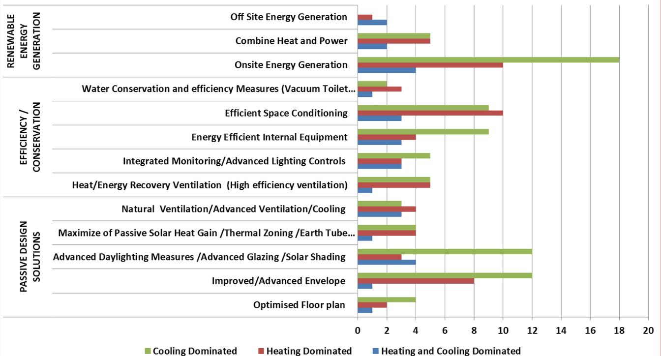
Figure 3. The whole-system approach to developing the solution sets for NetZEBs in various climates and an example of the solution set output.
