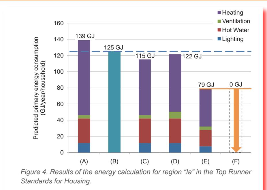
Figure 4. Results of the energy calculation for region "Ia" in the Top Runner Standards for Housing.
