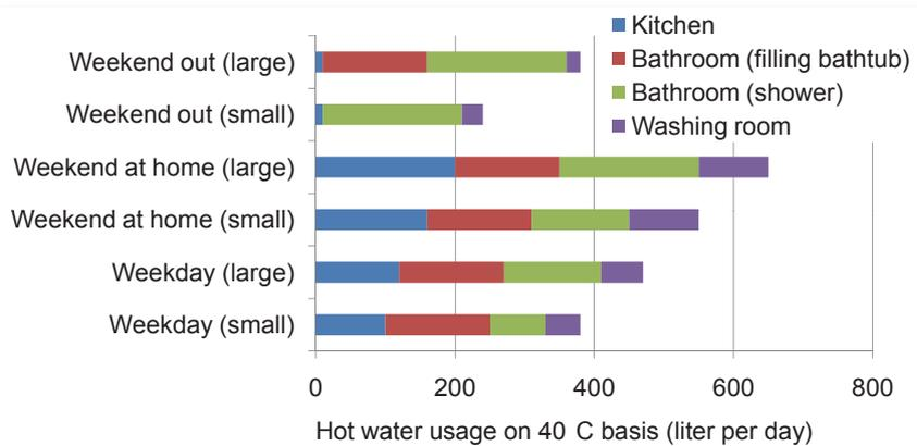
Figure 1. Domestic hot water usage pattern 'Corrected M-1 Mode' for 4-member family.
